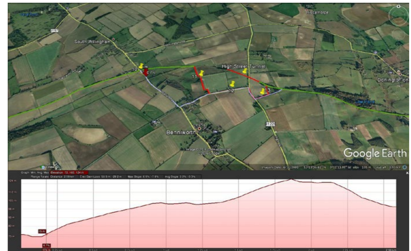
Figure 2. High Street Tunnel and environs showing gradient
